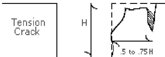
**B. SLIDING** or sluffing may occur as a result of tension cracks, as illustrated below.
