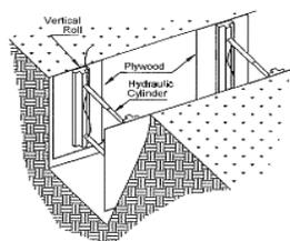
Vertical Aluminum Hydraulic Shoring (With Plywood)
