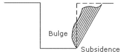
**E. HEAVING OR SQUEEZING.** Bottom heaving or squeezing is caused by the downward pressure created by the weight of adjoining soil. This pressure causes a bulge in the bottom of the cut, as illustrated in the drawing above. Heaving and squeezing can occur even when shoring or shielding has been properly installed.
