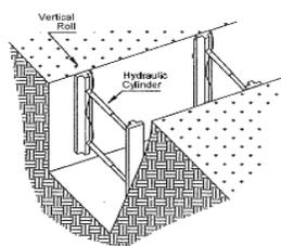
Vertical Aluminum Hydraulic Shoring (Spot Bracing)
