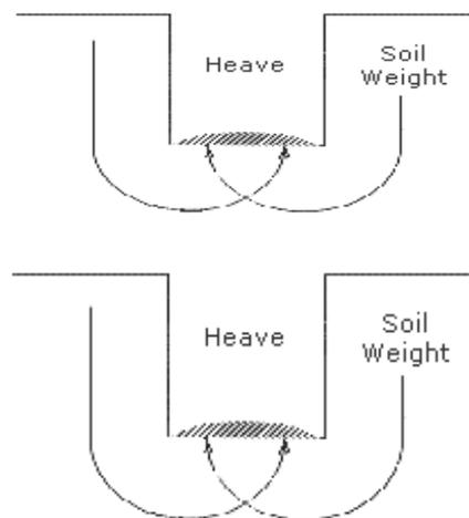
**F. BOILING** is evidenced by an upward water flow into the bottom of the cut. A high water table is one of the causes of boiling. Boiling produces a “quick” condition in the bottom of the cut, and can occur even when shoring or trench boxes are used.
