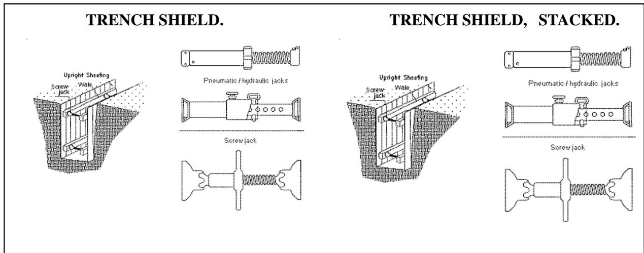
**COMBINED USE.** Trench boxes are generally used in open areas, but they also may be used in combination with sloping and benching. The box should extend at least 18 in (0.45 m) above the surrounding area if there is sloping toward excavation. This can be accomplished by providing a benched area adjacent to the box.
