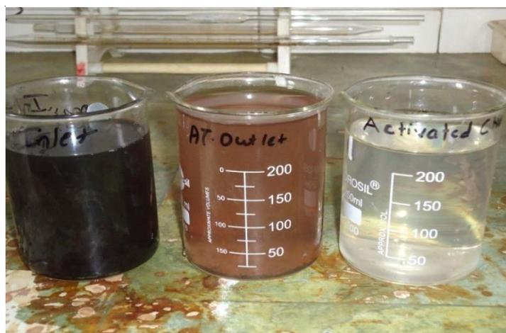
**Fig 2 : Colour reduction on using activated carbon**
