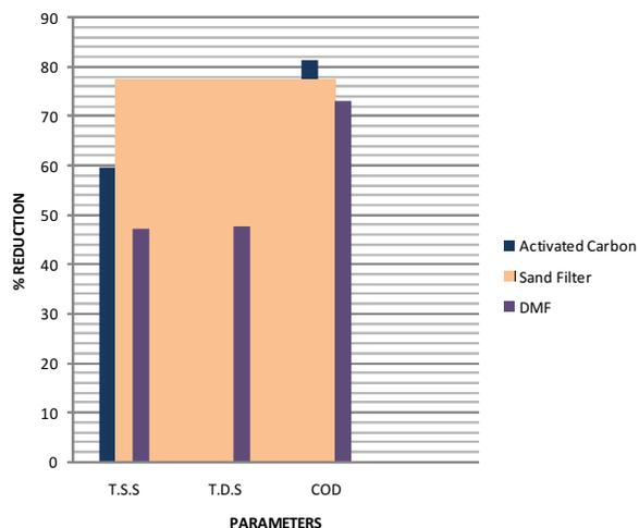
**Fig 3: Graphical Representation Of The Plant Performance**
